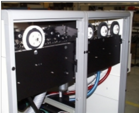
Fig.65b Gear train and drive motor position in processor.
