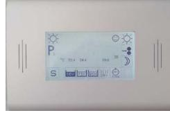
The control panel with a graphic interface will normally not require any intervention, but provides information about status. A film bar shows the position of films currently processing.
